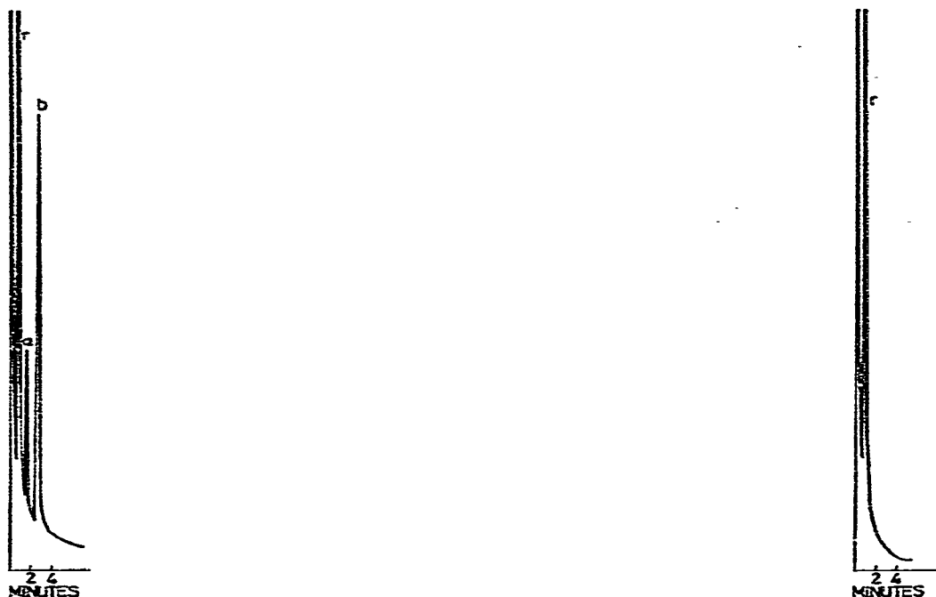
Fig. 1. Gas chromatograms of (a) n -octacosane (internal standard) and (b) piromidic acid methyl ester.
